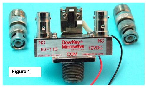
This was not a problem as I simply added 2 adapters, to convert the BNC females to SO-239. These coaxial relays operate on 12 Vdc and consume only 170 mA each (a total of 340 mA) when activated.
