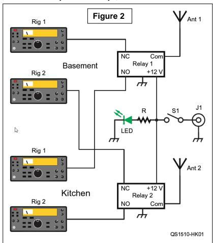
one relay is connected to the 220 MHz antenna and the common of the other to the dual-band antenna. The NC output of each relay is connected to the basement rigs, and the NO outputs are connected to the kitchen rigs. The LED in fig 2 can be any you have available: Size resistor R to match the particular LED you use.
