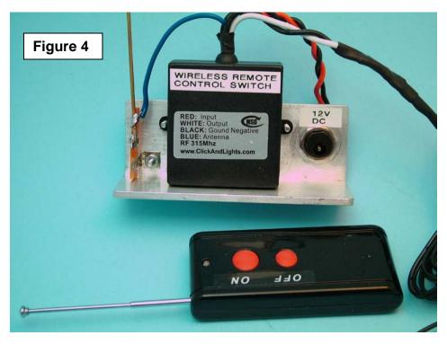
Another point to consider is that some wireless switches are toggle types with only one button on the wireless remote control, that is, when the switch is off. pressing the button will turn it on; if the switch is on, pressing the button will turn it off. Others have ON separate and OFF buttons. I prefer this type because you can press the OFF button anytime you forget the state of the switches.
